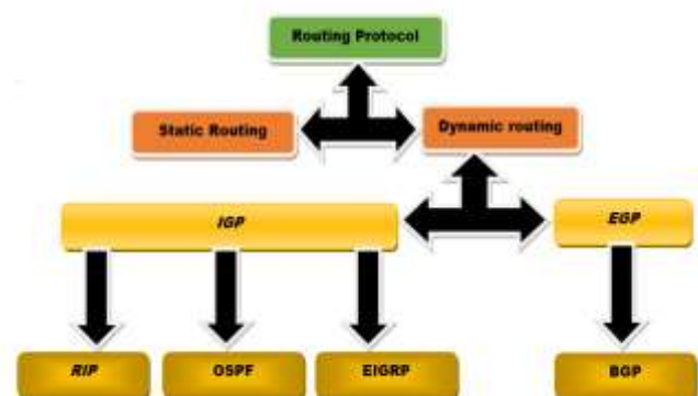
Figure1: Classification of Dynamic Routing protocol
