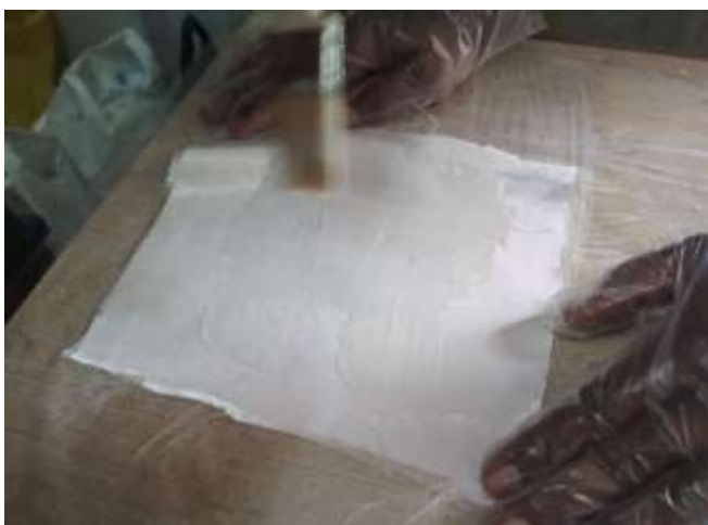
Figure 3.1: Fabrication by hand lay-up technique (compression)
