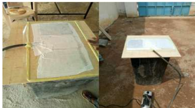
Figure 3.1.1: Vacuum bagging of composite
