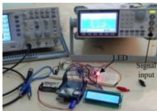
Figure 3: Setup, measurement and testing Arduino Uno output
