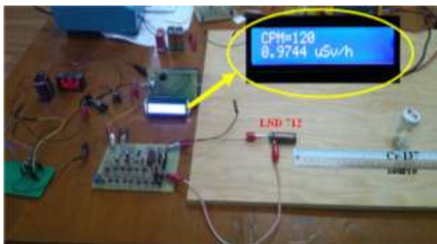
Figure 8: Experimental set up of Arduino based GM counter
