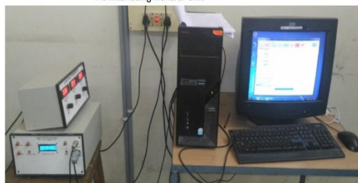
Lathe Tool Dynamometer PC Interfacing Setup
