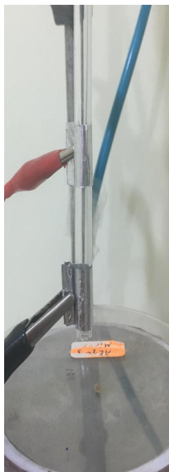
Double-ring electrode configuration with wall thickness of 1mm
