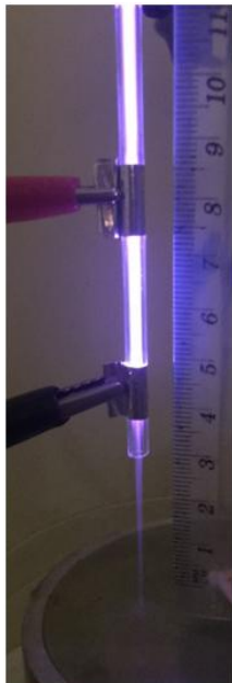
Double-ring electrode configuration with wall thickness of 0.80mm
