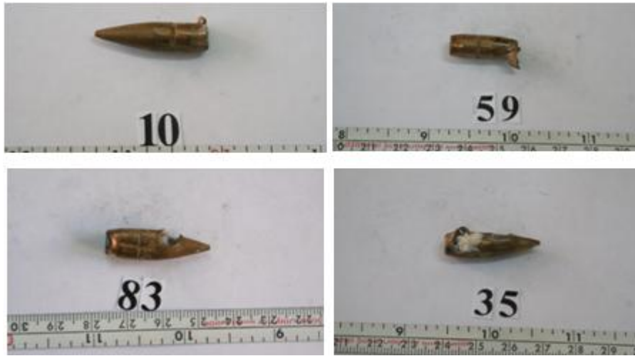
Figure 2: Showed the distorted bullets of 7.62x51(SLR) mm and .303” calibre.
