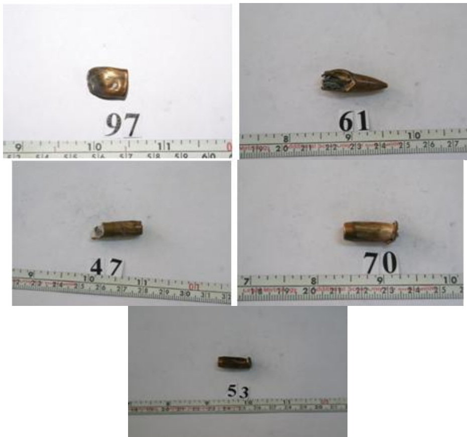
Figure 3: Showed the distorted bullets of 9mm and 7.62x39 (AK-47) mm calibres
