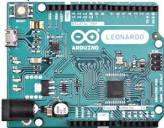
Figure 4: Arduino Leonardo board
