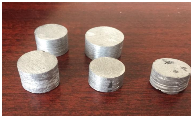
Figure 4.3: The Specimens prepared for Hardness test
