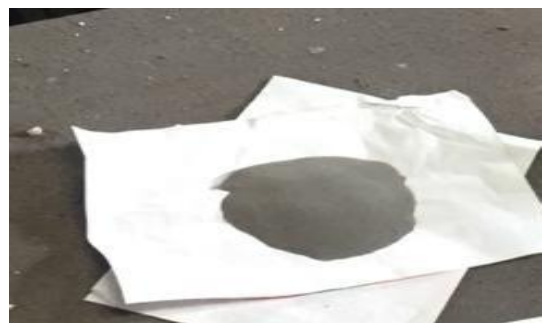
Figure 2.1: Stainless Steel 316 Powder (45 micron)
