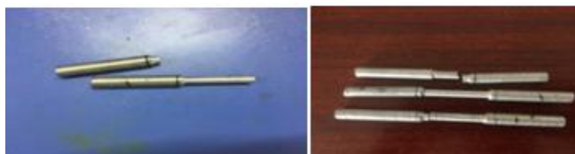
Figure 4.6: The breakage specimens after tensile testing
