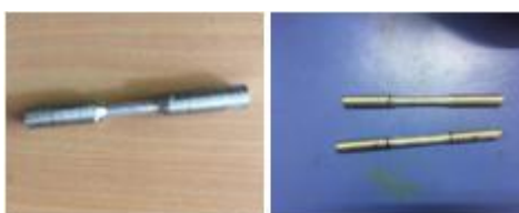
Figure 4.5: Specimens after machining on lathe
