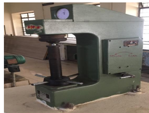
Figure 4.2: Brinell hardness testing machine.
