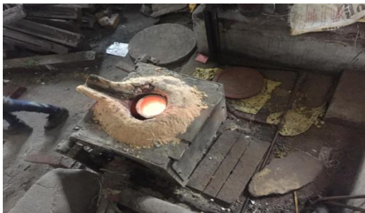
Figure 3.1: Heating aluminium alloy 6061 in furnace
