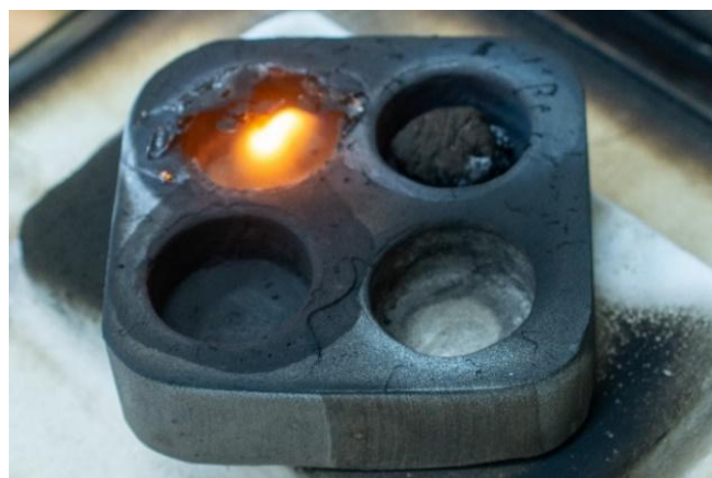
Figure 11: Structural changes of the samples at 550°C.
