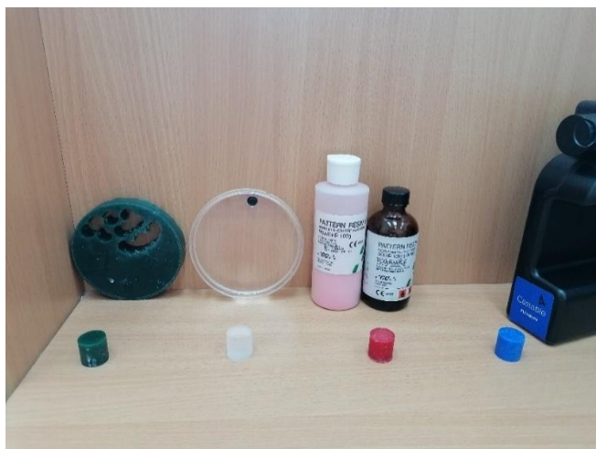
Figure 1: The examined samples are shown, from left to right as follows: CAD/CAM wax (Yeti Dental ™ ), C-cast ® (KaVo Dental ™ ), Pattern resin LC ® (GC ™ ), and Castable Resin ® (Formlabs ™ )
