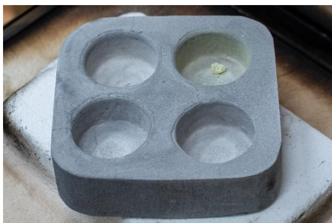
Figure 13: Residual ash remnants amount reduction at 1050°C.
