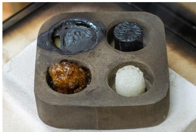
Figure 9: Structural changes of the observed samples at 400°C.
