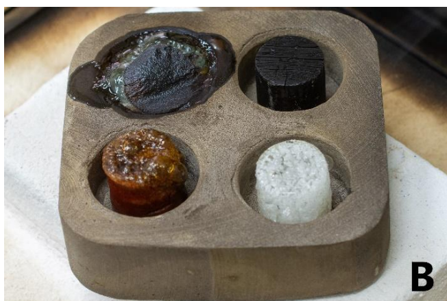
Figure 8: Structural changes of the observed samples at 350°C, before (A) and after (B) the 10 minutes holding.
