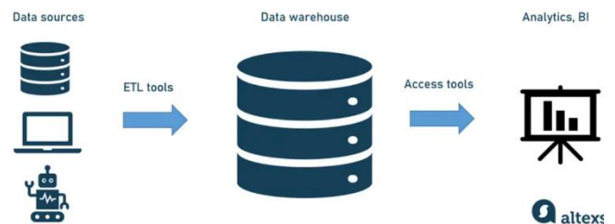
Figure 11: Data warehouse structure.
