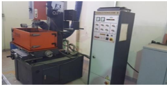
Figure 3: RoboForm 2-LC spark EDM Machine
