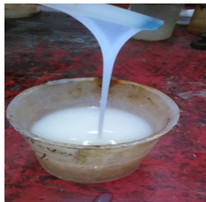
Figure 2: Laminating dispersive adhesive
