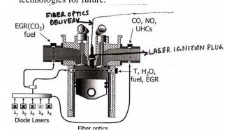
Above diagram is a hypothetical representation of both laser ignition and optical laser sensors
