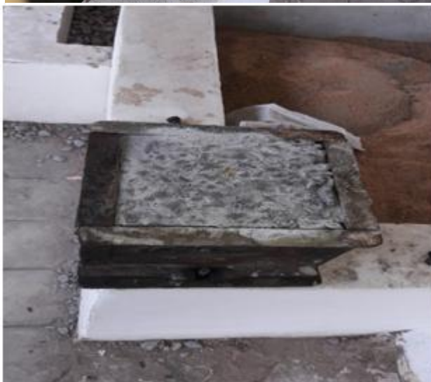
Fig:- Cube Test Of Waste Glass
