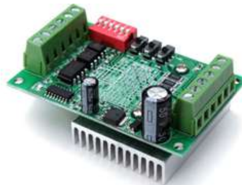
Figure 4: (5)TB6560 driver board
